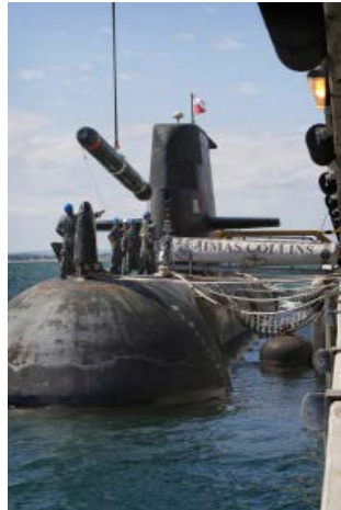
A Submarine Launched Countermeasure Emulator (SLACE) vehicle is embarked onto HMAS Collins from Diamantina Pier at HMAS Stirling.
