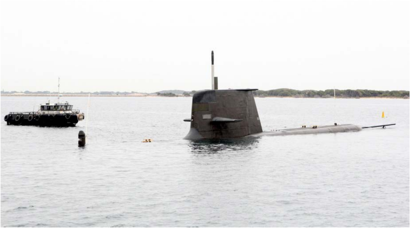
HMAS Waller conducts a dive incline trial at Fleet Base West.
