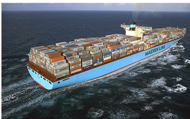
Figure-1 Emma Maersk requires gantry cranes capable of handling movements over 23 TEU rows. Source: www.gcaptain.com
