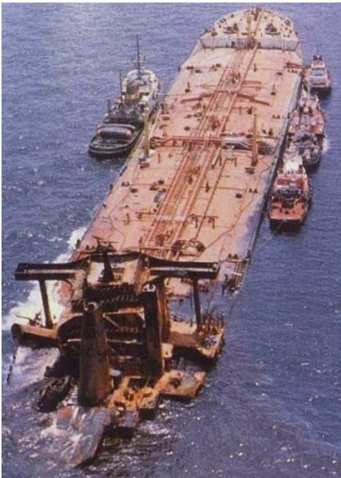
Figure 2. ULCC Bridgeton (400,000 dwt) under tow after hitting an Iranian mine west of Farsi Island on 24 July 1987. [weblog.leidenuniv.nl/fdr/1948/Bridgeton]
