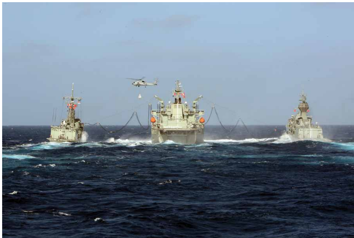
The surface force of Exercise TRITON FURY conduct a dual-RAS and vertical replenishment with a Seahawk helicopter off the West Australian coast.
