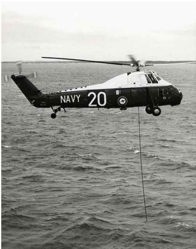
A Westland Wessex 31A with its dipping sonar deployed during an anti-submarine exercise
