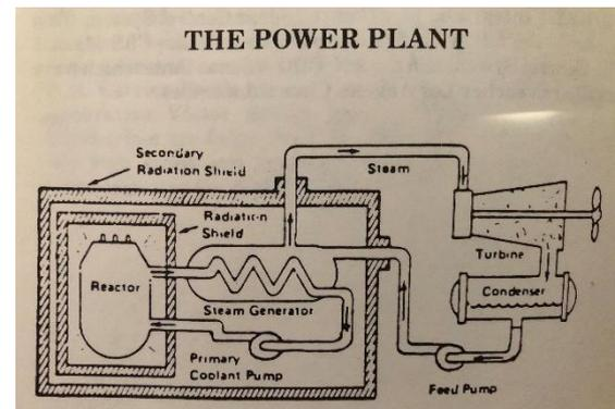
A basic diagram of the two separate closed systems that interact to propel a submarine through the water.
