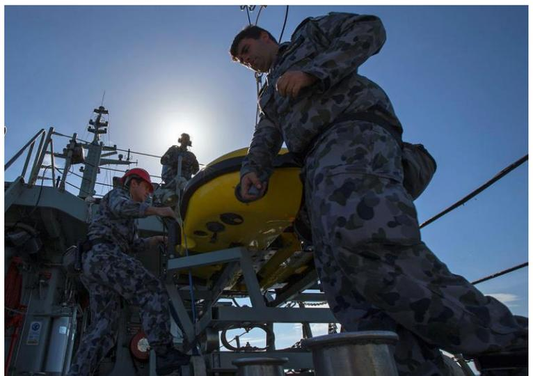
HMAS Huon personnel prepare to launch the Double Eagle Unmanned Underwater Vehicle to inspect a potential mine contact during the Mine Counter Measures and Diving Exercise 2014.
